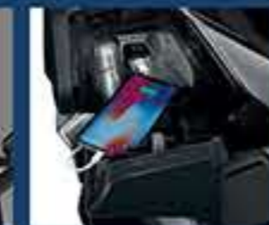
Console Box with Power Charger
